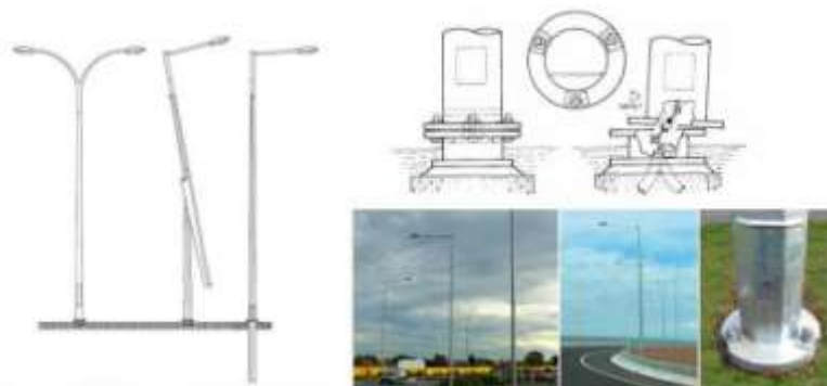
A4.Figura 21:Stâlpi de tip “rupere de la bază” (Source: Department of infrastructure, Energy and Resources: Road Hazard Management Guide, Tasmania, 2014)
